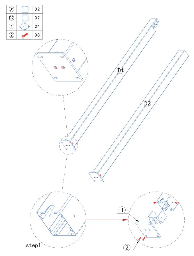
1. Loosen screws from post hardware on the post D1 、 D2 , attach Beam C to the D1 、 D2 , then use screws to fasten.
