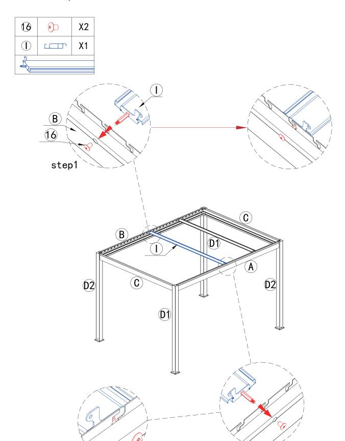
1. Fit all common louvers G X21 for 300x300cm and G X30 for both 300x400 into the remaining slots in the beams.
