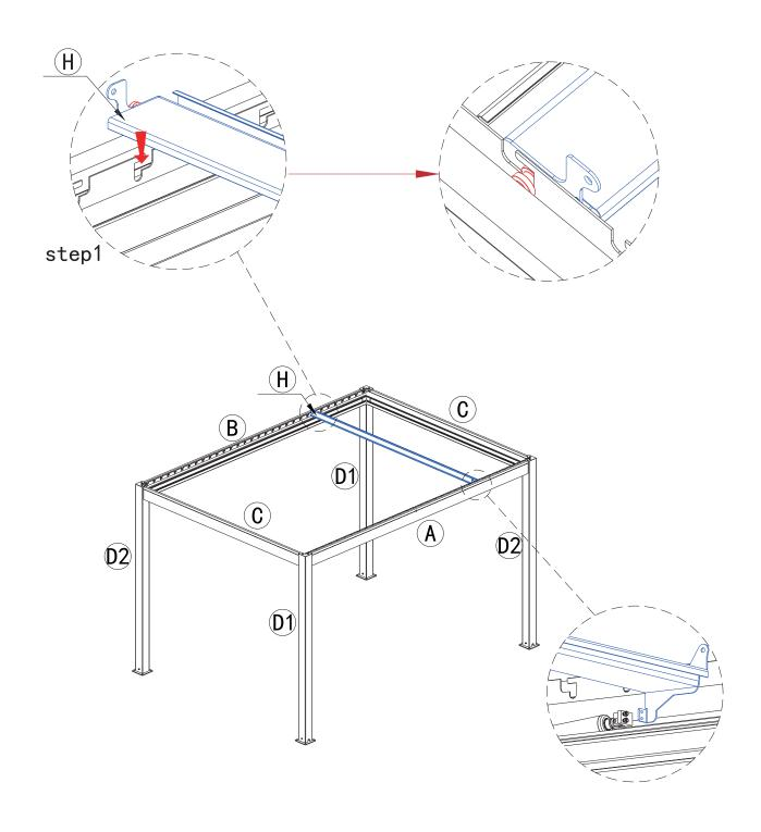
1.Place centre louver  $\fbox{I}$  in the middle slot on the beam  $\fbox{A}$  and  $\fbox{B}$ . Using  $\fbox{16}$  X2, secure the louver in place .
