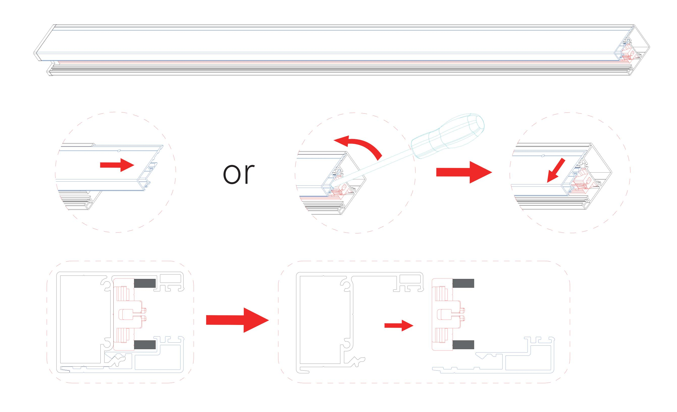
Remove the cover plate and inner track successively
